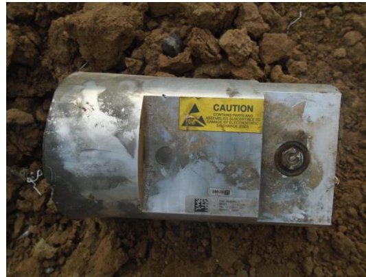
Fig.4 Control Actuator System (CAS) of a GBU-69/B. © SOMALIMEMO
