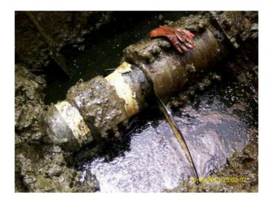
In another case, a spill occurred at Ikarama in Bayelsa state on 24 May 2013. The JIV, which took place on 30 May, six days later, found the spill was due to a hacksaw cut. 64 However, the photograph (reproduced above) does not show a hacksaw cut. According to Accufacts: "Most likely this photo suggests that the seal on a previous clamp repair has failed for various reasons, such as poor installation." 65
