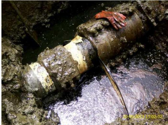
In another case, a spill occurred at Ikarama in Bayelsa state on 24 May 2013. The JIV, which took place on 30 May, six days later, found the spill was due to a hacksaw cut.<sup>64</sup> However, the photograph (reproduced above) does not show a hacksaw cut. According to Accufacts: “Most likely this photo suggests that the seal on a previous clamp repair has failed for various reasons, such as poor installation.”<sup>65</sup>
